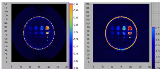
Fig. 2. Image reconstruction results by EM(left) and TV(right).
