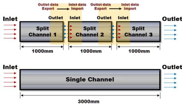
Fig. 2 Graphical explanation for split channel method
