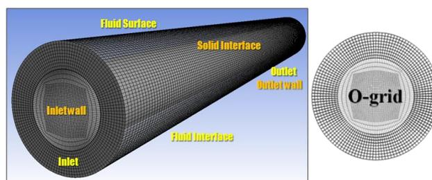
Fig. 1 Grid systems for singular rod
