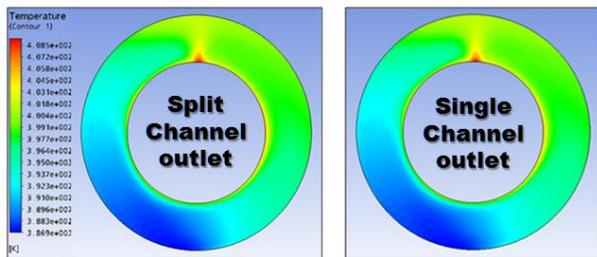
Fig. 3 Comparison of outlet temperature distribution
