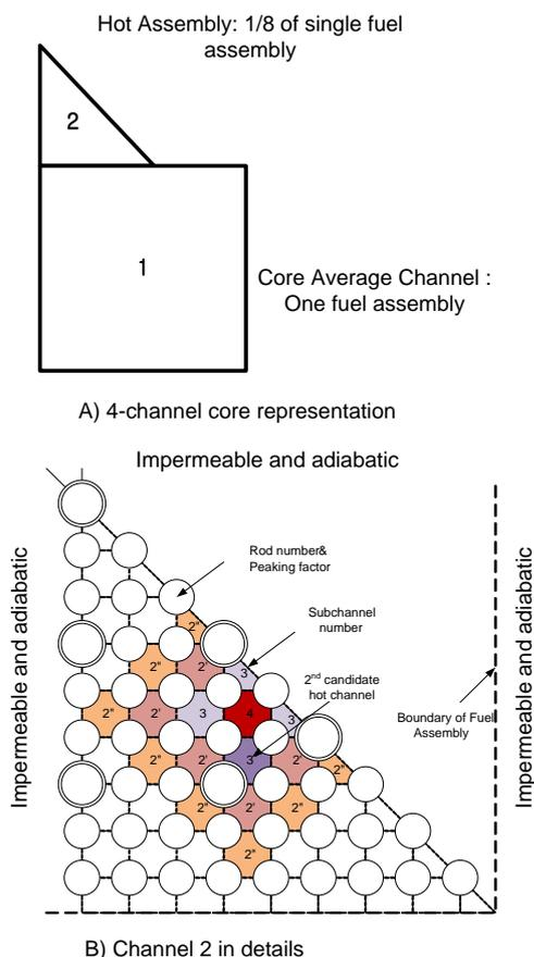
Fig. 1. 4-Channel lumping model of FAST code to calculate the DNBR in hot channel.
