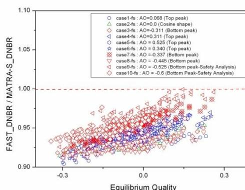
Fig. 2. Comparisons of MDNBR of FAST and MATRA-S for 10 axial power shapes.
