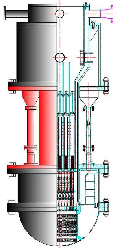
Fig. 2. Schematics of SMART Reactor Simulator
