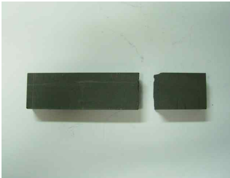
Fig. 4 Fracture shape of graphite IG-11 and IG-110
