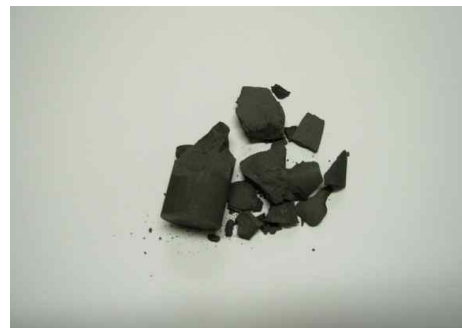
Fig. 2 Fracture shape of graphite IG-11 and IG-110
