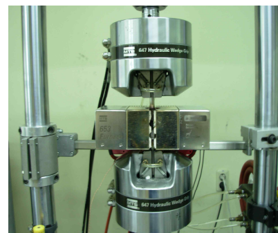
Fig. 2 Experimental setup with heating chamber.
