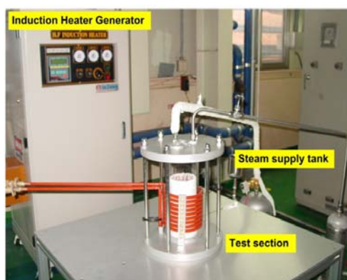
Fig. 2. Photograph of the layer inversion test facility.
