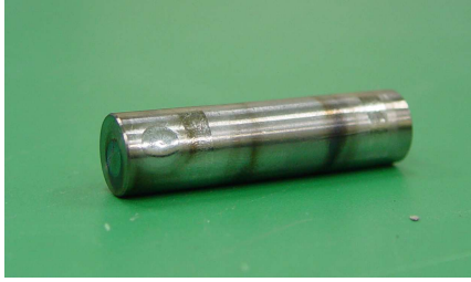
Fig. 3 The zry-4 tube contained a fuel sample
