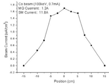
Fig. 3. Cobalt beam profile on target measured by a Faraday Cup
