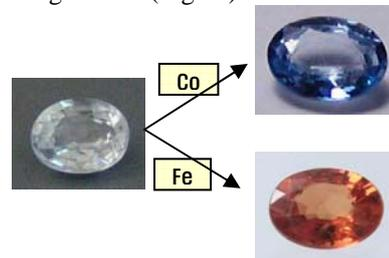
Fig. 4. The Changes of sapphire color by cobalt and iron ion implantation (100keV)
