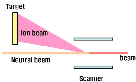
Fig. 2. A schematic of charged particle trajectory by electrostatic scanner
