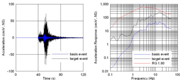
Fig. 1. Acceleration seismograms (left) and response spectrums (right) of the basis and target event. The DRS of the Uljin NPP site is also depicted.
