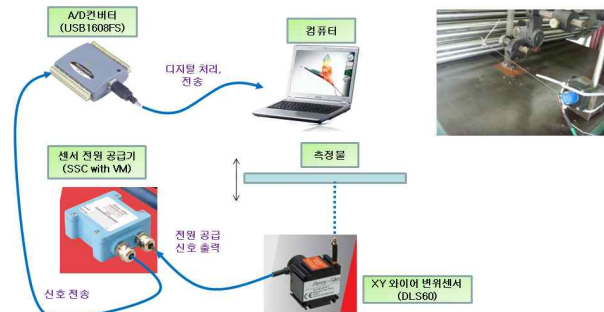
Fig. 1 Layout of wire amplitude measurement system
