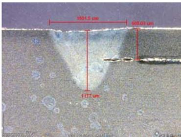
Fig. 3. Macro-section of a laser welded specimen
