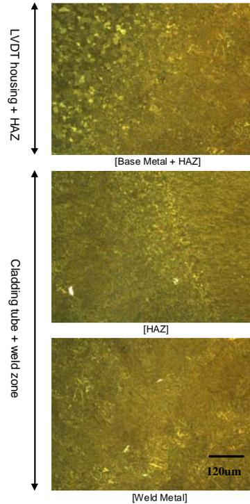
Fig. 4. Microstructure of a Zircaloy-4 welded specimen
