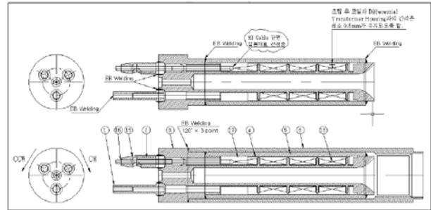
Fig. 1. Configuration of LVDT tube and housing specimen
