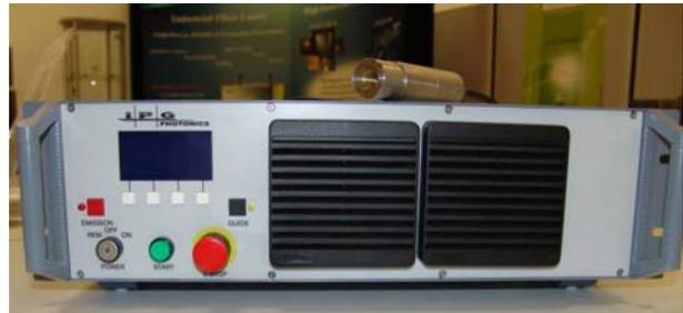
Fig. 2. Photography of a laser welding machine
