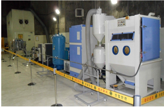
Fig. 2. The dry abrasive blasting equipment
