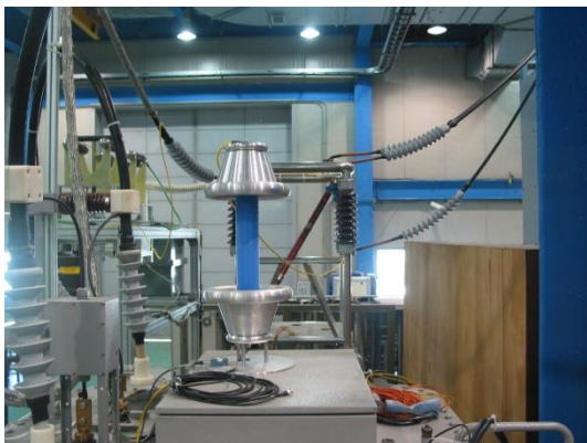
Fig. 5. Installation for measurement of the mod-anode voltage
