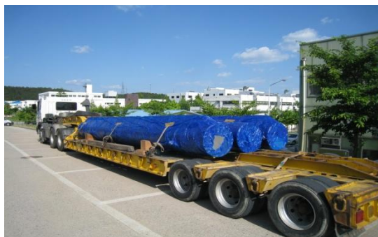
Fig. 1: 100MeV DTL tanks movement
