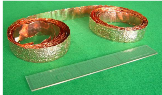
Fig. 4. Cu Foil produced by roll casting
