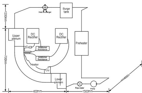
Fig 1. Schematic diagram of the experimental loop
