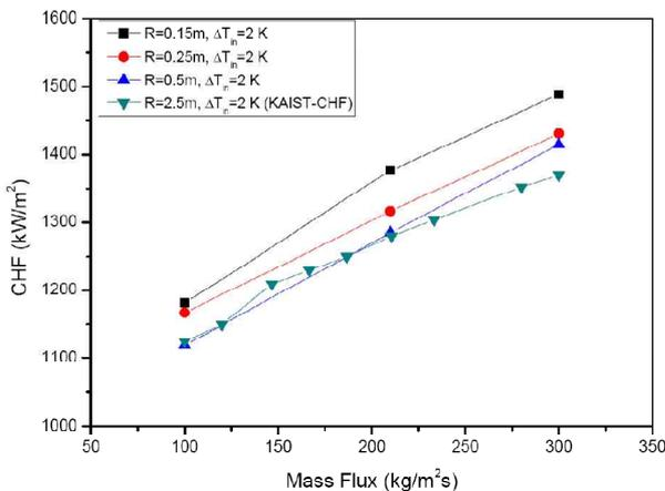
Fig 3. CHF data according to mass flux
