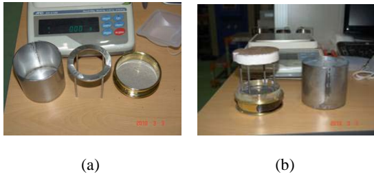
Fig. 1. Photographs of (a) a sieve assembly for the solid-liquid separation and (b) a frozen LiCl-KCl salt collected in the bottom container.
