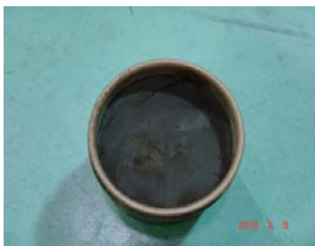
Fig. 2. Photograph of the salt (LiCl-KCl- UCl_3 ) residue on the sieve after the solid-liquid separation experiment.
