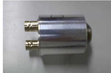
Fig. 2 Photograph of the transmit-receive EMAT sensor
