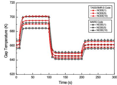
Fig. 3. Gap Temperature Variation along the time.
