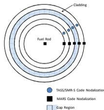
Fig. 2. Fuel rod nodalization to the radial direction.
