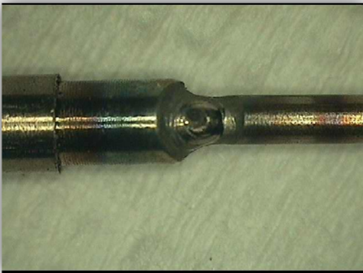
Fig. 2 Photograph of a busing/MI cable sheath specimen welded by using a micro-TIG welder
