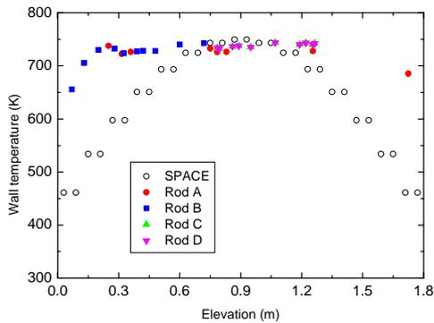
Figure 3. Distribution of wall temperature with respect to elevation at the moment of water injection for reflow.
