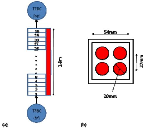
Figure 2. (a) SPACE nodalization and (b) configuration of rod bundle.
