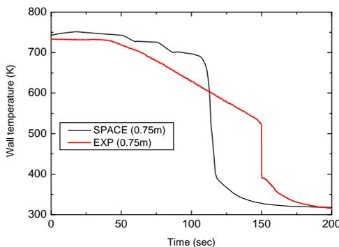
Figure 4. Time variation of the wall temperature at elevation of 0.75m from the bottom.
