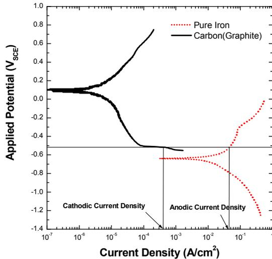
Fig. 2. Potentiodynamic polarization curves obtained for pure iron and carbon (graphite) in a  $\text{FeS}+\text{HCl}+\text{Na}_2\text{SO}_4$  solution with a scan rate of  $0.5\text{mV/s}$ .
