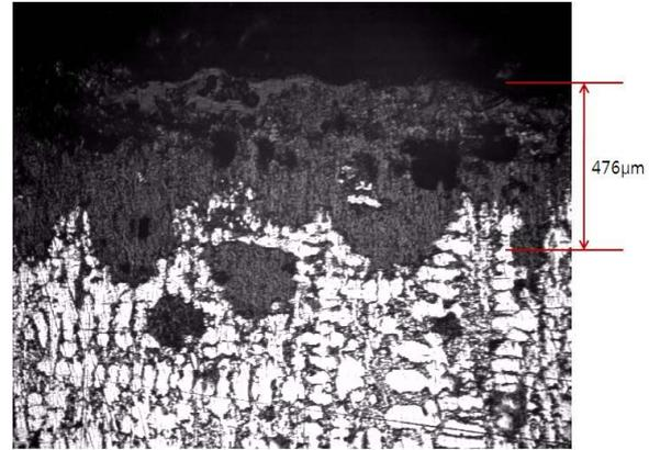
Fig. 3. Cross-sectional view of optical micrograph for gray cast iron (GC250), selectively leached for 30 hours in a  $\text{FeS}+\text{HCl}+\text{Na}_2\text{SO}_4$  solution at  $75^\circ\text{C}$ .
