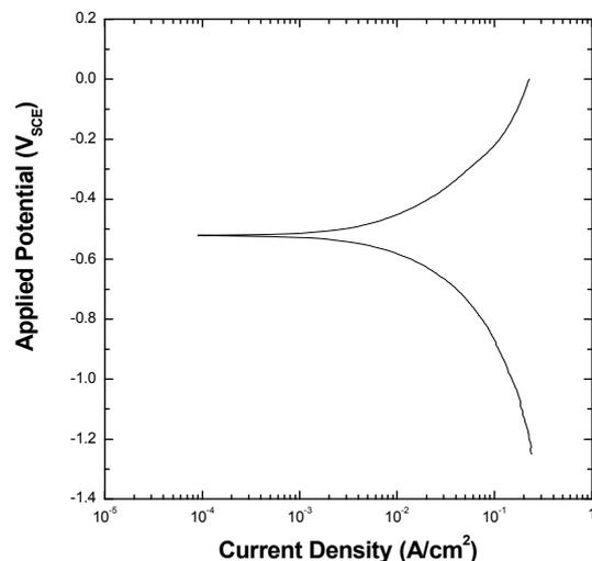
Fig. 1. Potentiodynamic polarization curve obtained for gray cast iron, GC250 in a FeS+HCl+Na<sub>2</sub>SO<sub>4</sub> solution with a scan rate of 0.5mV/s.
