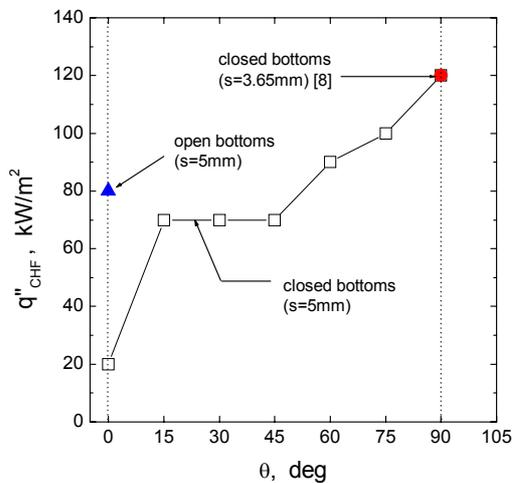
Fig. 2. Changes in the CHF with the inclination angle.
