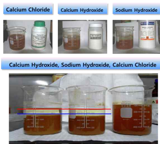
Fig. 2 Precipitation experiment of uranium leachate with cohesive agent
