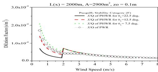
Fig. 5 Change of atmospheric dispersion factor for PHWR with  $\theta_L$  change
