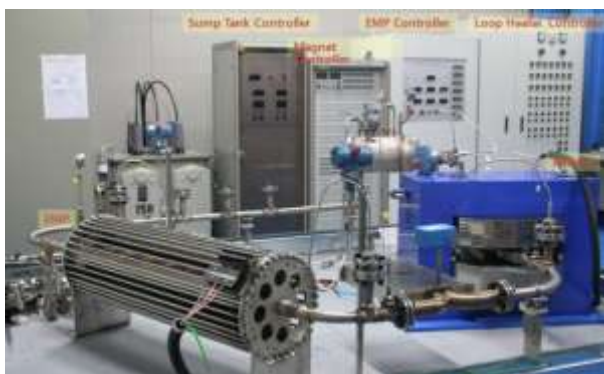
Figure 1. PbLi circulation loop under construction in KAERI(ELLI).
