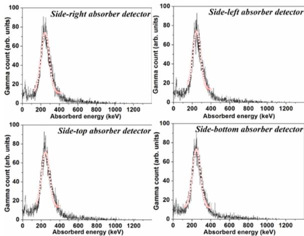
Fig. 2. Energy distributions deposited in side absorbers.
