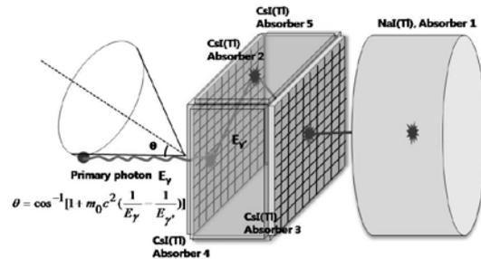
Fig. 1. Double-scattering Compton camera with side absorbers.
