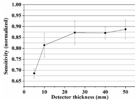
Fig. 3. Imaging sensitivities as a function of thickness of the side absorber.
