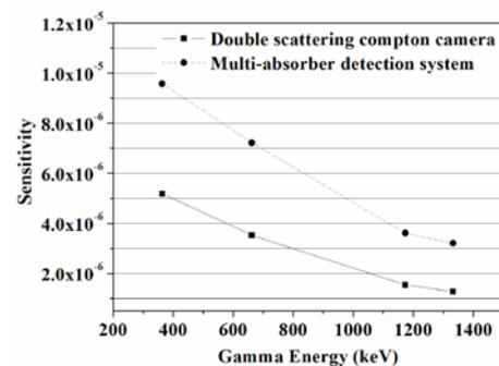
Fig. 4. Imaging sensitivities of DOCI as a function of the photon energy with and without side absorbers.
