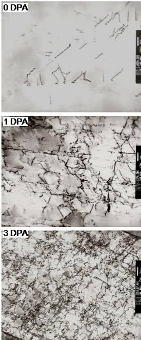
Fig. 2 Variations of the dislocation density depending on the proton irradiation dose.
