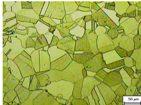
Fig. 1 OM image of the un-irradiated specimen.
