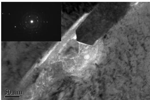
Fig. 4 TEM bright field image of corrosion products and the related selected area diffraction pattern
