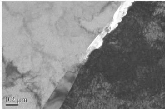
Fig. 3 TEM bright field image of a PWSCC crack in Alloy 600
