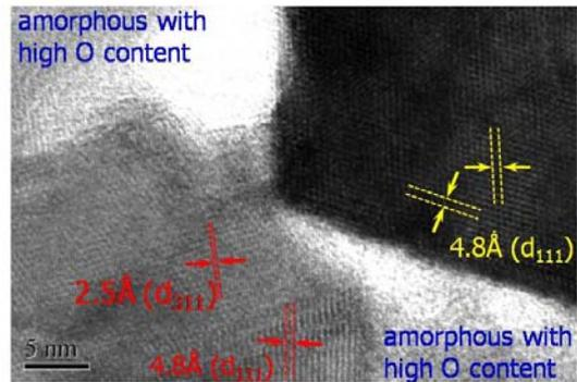
Fig. 5 High resolution image of oxides in a PWSCC crack of Alloy 600
