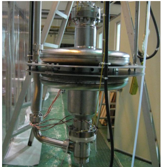
Figure 1. Two-cell SRF cavity installed in the insert.
