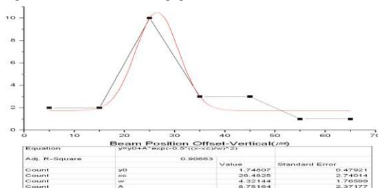
Fig. 5. The distribution of vertical beam displacement from beam pipe center.
