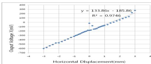
Fig. 1. Sensitivities of LR-BPM Electronics for horizontal direction.
