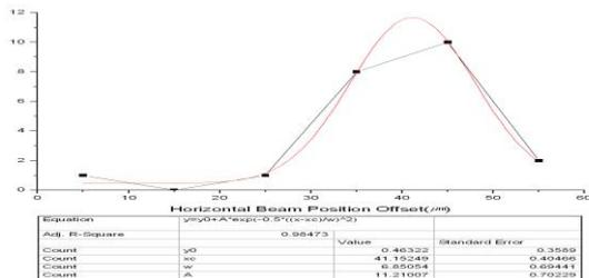
Fig. 4. The distribution of horizontal beam position displacement from beam pipe center.
