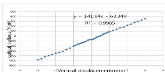
Fig. 2. Sensitivities of LR-BPM Electronics for vertical direction.
