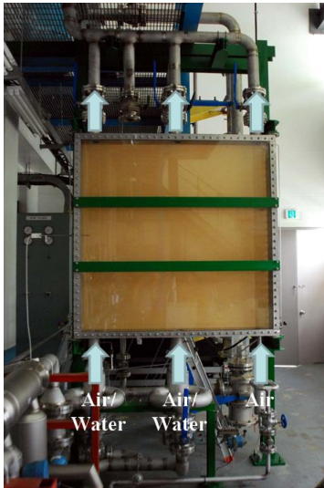
Fig. 2. Photograph of test facilities and definition of inlet and outlet nozzles.
