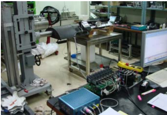
Fig. 3. Data Acquisition using K-AUT System
