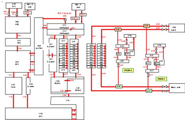
Figure 2 Nodalization of SMART system for SBLOCA with MIDAS/SMR
