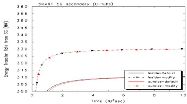
Figure 1 Predicted thermal power of SMART
