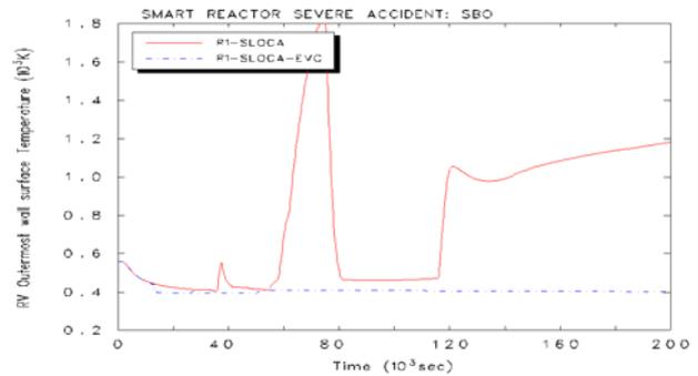
Figure 3 Outer surface of lower head temperature with and without EVC (external vessel cooling)
