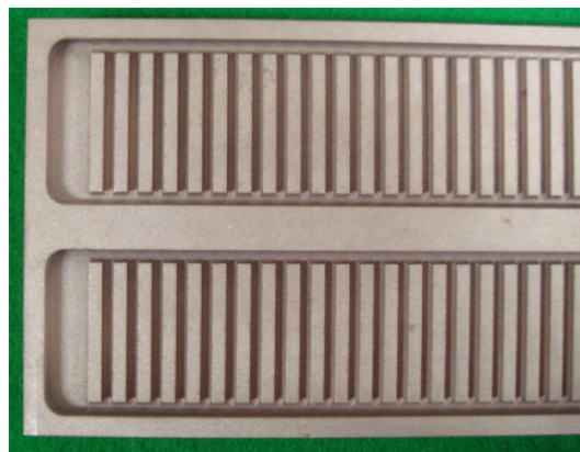
Fig. 2. Fabricated Cu-alloy heat sink prior to the bonding, which has a hypervapotron type cooling channel.
