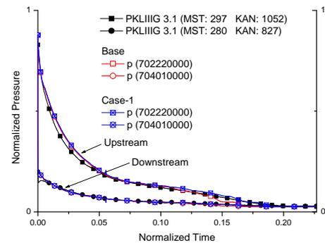
Figure 2. Upstream and downstream pressure of break orifice
