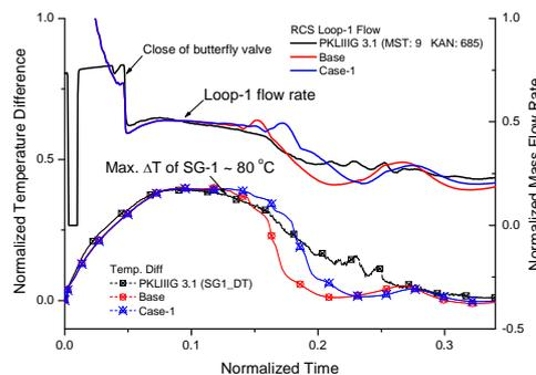
Figure 3. RCS flow rate and  $\Delta T$  of SG in affected loop
