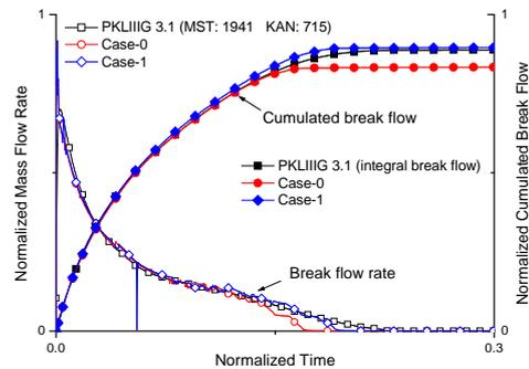
Figure 1. Break flow rate and mass
