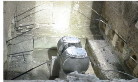
Figure 2. Test model installed in the furnace.
