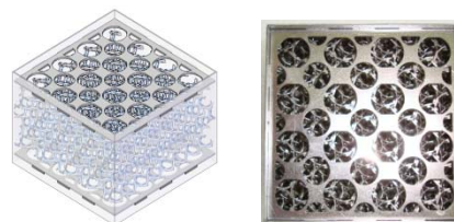
Fig. 2. Schematic and mockup view of the perforated plate structure for segmented fuel rods.
