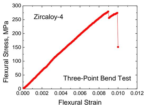
Fig. 3. Flexural stress and strain of Zircaloy-4 during a three-point bend test.
