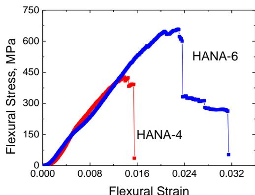
Fig. 4. Flexural stress and strain of HANA4 and HANA-6 during a three-point bend test.
