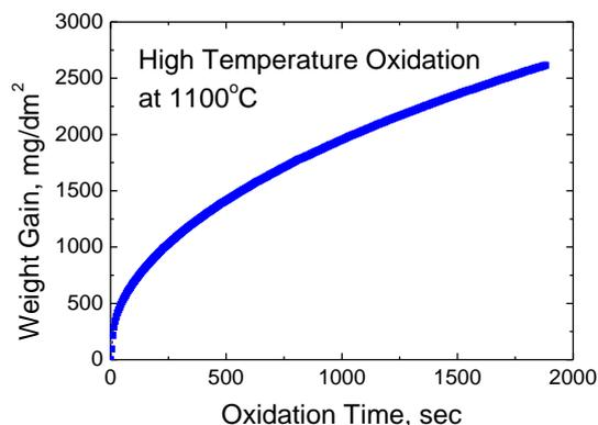
Fig. 2. High temperature oxidation of Zircaloy-4 at 1100°C
