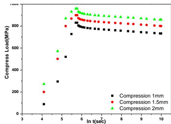
Fig. 1. Variation in compressive stress depending on time at room temperature
