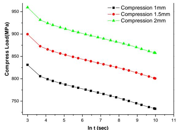
Fig. 2. Stress relaxation with time for successive runs at room temperature
