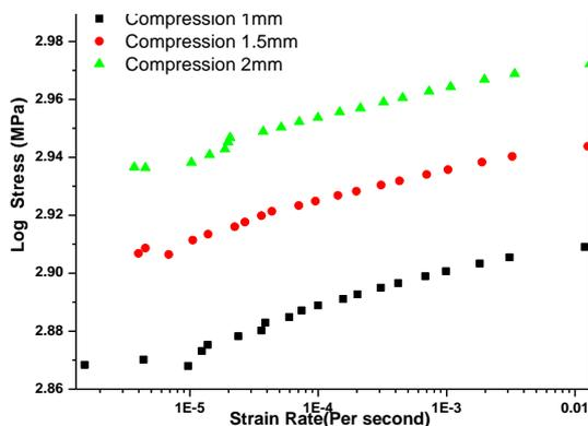
Fig. 4. Stress to strain rate curve at room temperature
