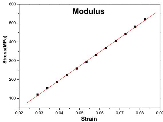
Fig. 3. Compressive stress-strain curve for sample deformed by 1mm at room temperature
