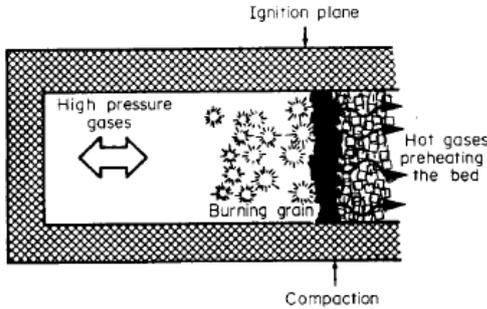
Fig.1. A schematic of flame spread in a highly confined column of explosive [2]
