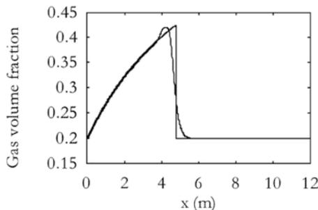
Fig.2 Gas volume fraction at time 0.4 s. (exact solution; bold lines).
