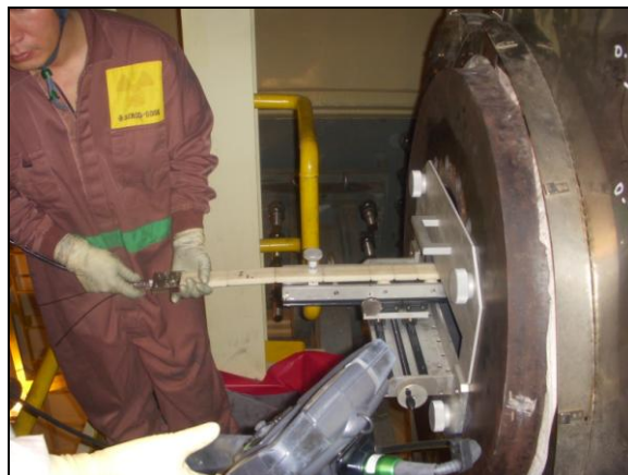
Fig.2 Visual Inspection System
