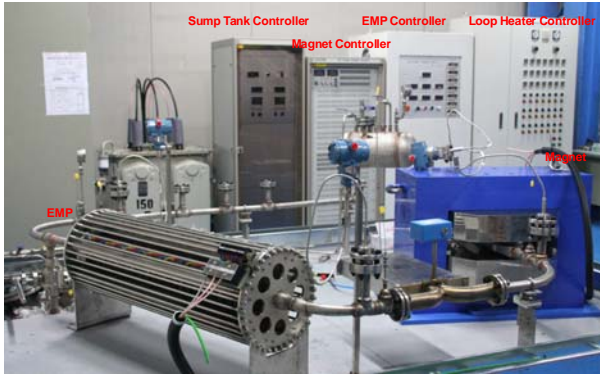
Fig. 4. Experimental loop of the PbLi liquid breeder.
