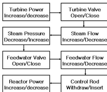
Fig. 1 Control Logic for turbine-leading strategy
