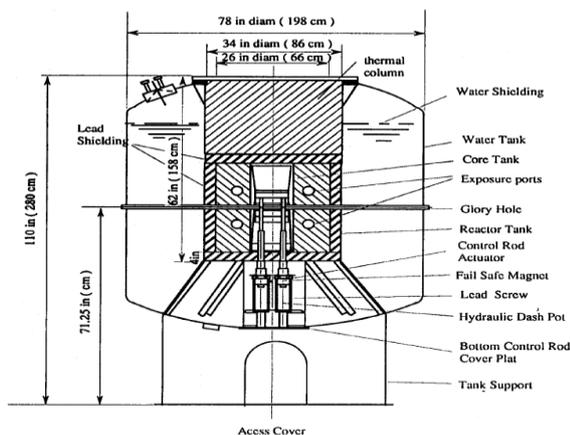
Figure 1. Structure of AGN-201K reactor
