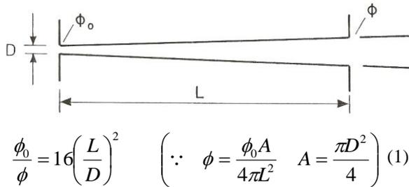
Figure 3. Divergent-Beam Collimator
