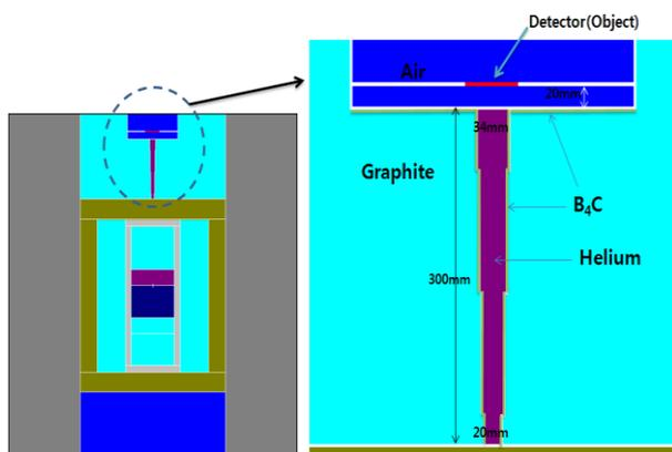
Figure 4. Collimator modeling
