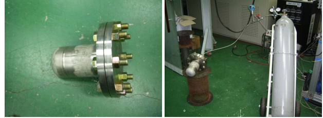
Figure 4. the assembled zig Figure 5. leak test equipments
