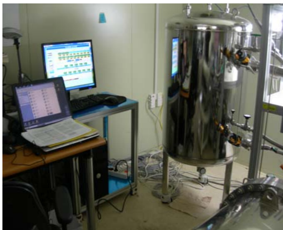
Fig. 1. A 260L tank and data acquisition system
