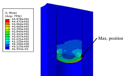
Fig. 3 Deformed shape and stress contour of the fuel plug on which maximum stress was developed
