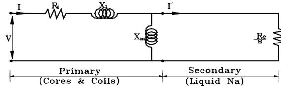
Fig. 2. The equivalent circuit for an EM pump design
