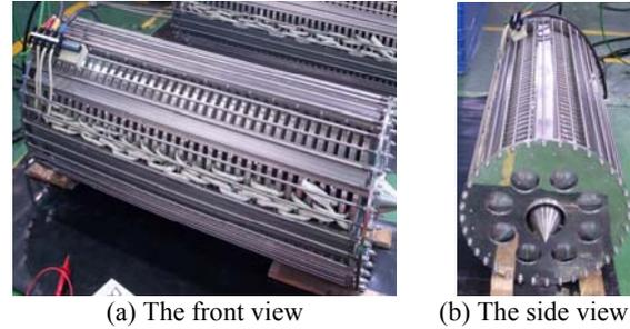
Fig. 2. The completed annular linear induction EM pump
