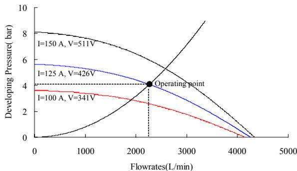
Fig. 3. P-Q characteristic of the designed EM pump by the theoretical calculation
