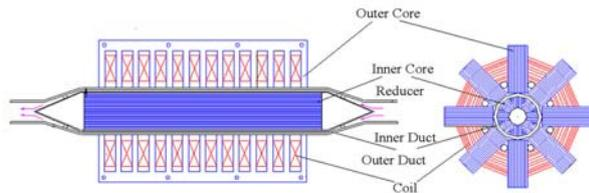
Fig. 1. Cross-sectional view of the annular linear induction EM pump
